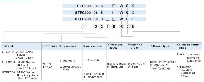
$[Note1] \ \ The\ maximum\ work\ pressure\ of\ lower\ pressure\ type\ is\ 0.4 MPa (58 psi);\ [Note2]\ Please\ refer\ to\ page\ 194\ for\ details\ of\ reflux\ valve.$
